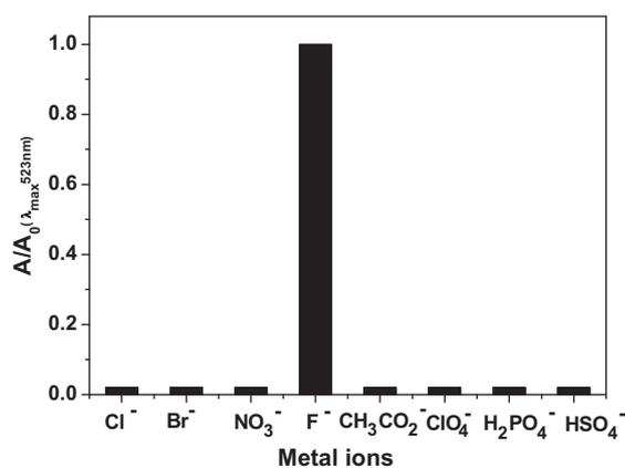
**Fig. 3.** Comparison of absorption ratio of dye **3** with various anion detections, where  $A$  and  $A_0$  represent the absorbance in the presence and absence of anions, respectively.
