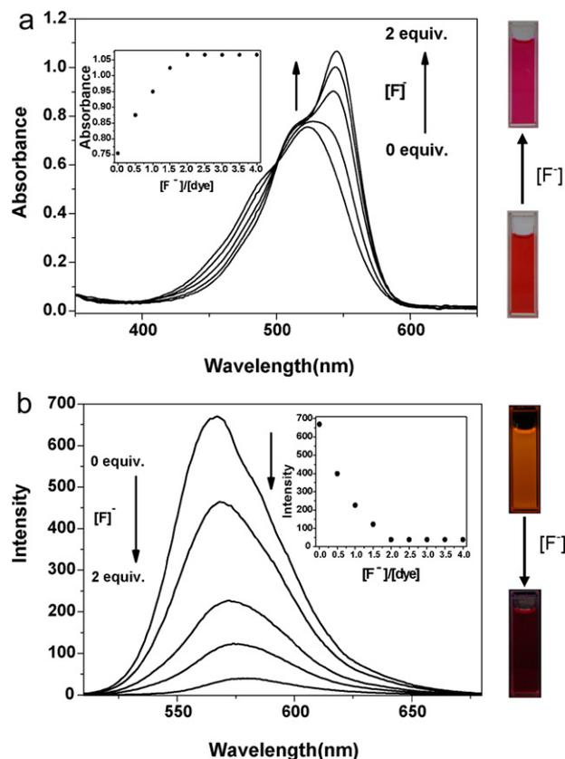
Fig. 2. Absorption (a) and emission (b) changes of dye **3** ( $1 \times 10^{-5} \text{ mol}$ ) in  $\text{CH}_3\text{CN}$  with fluoride.
