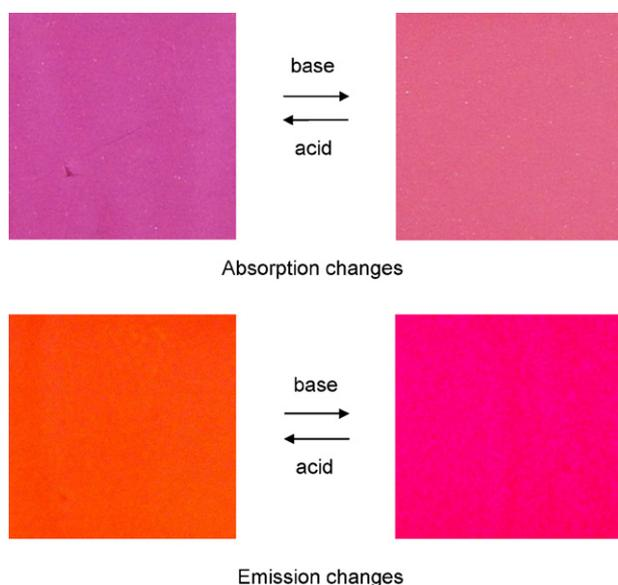
**Fig. 7.** Color changes with absorption and emission of dye sensor casted on thin layer silica gel sheet in acid/amine VOCs exposure.
