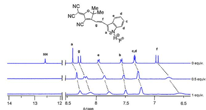
**Fig. 4.** <sup>1</sup>H NMR spectral change with strength of intermolecular proton transfer between NH fragment and fluoride.
