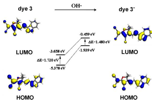
**Fig. 5.** Electron distribution of HOMO and LUMO energy levels of dye **3** and dye **3a**<sup>-</sup>.
